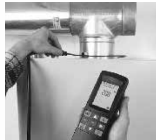
Storable O 2 air inlet measurement for ambient air-dependent systems (only testo 325 XL)
