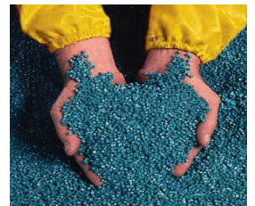
Granulate drying: dry air is a requirement for product quality
