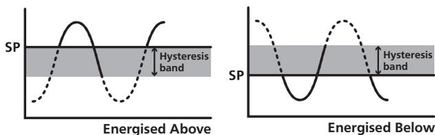
***CTRL - SP VALUE** controls setpoint deactivation point. **HYSTERESIS VALUE** controls setpoint reactivation point.*
