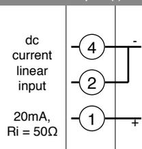
• Linear input with 2-wire transmitter
