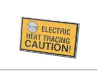
**CL...**vinyl-based peel-and-stick caution labels are intended for direct exposure to industrial environments. Electrically heated pipelines and vessels should be clearly identified at frequent intervals along the pipeline or vessel. Caution labels should be placed at 3 to 6-m intervals or as required by code or specification. Additional languages or other texts are available; contact Thermon.
