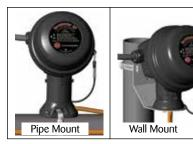
Terminator ZP... is designed to fabricate power connections, in-line/T-splice connections or for making end terminations. The Terminator ZP-XP is suitable for use in hazardous areas (Ex e T6/T4), harsh industrial environments and has a IP66 rating. The upfront positioning of the terminal block permits easy access during assembly and for future routine maintenance.
