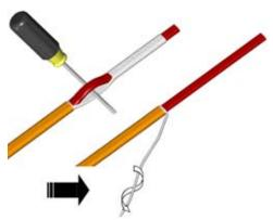
Separate braid strands and pull cable through opening in braid. Twist braid into a pigtail. Trim ends of braid.
