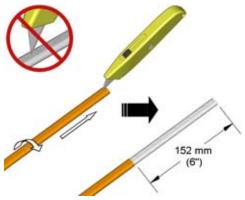
Cut and remove overjacket. Do not cut metallic braid.
