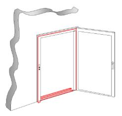
Warm air entering a cool room will condense and freeze upon contact with a cold surface.
