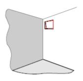
These are mounted in the cool room wall and used to maintain normal atmospheric pressure allowing air to enter or exhaust as required.
