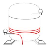
Compressors may be damaged by the formation of refrigerant liquid in the crankcase particularly after long 'off' periods.
