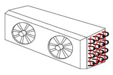
Defrost heaters in evaporators may not always extend to the bends, and therefore these may be traced with heater cables to assist the defrost operation.
