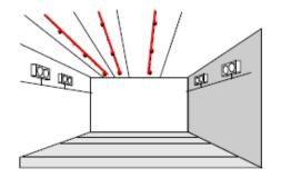
Where these are installed in cool rooms trace heating will be required to prevent freezing on exposed pipe work and fittings.
