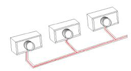
The drain line from the drip trays also requires heat tracing to prevent ice formation. The heater may be attached to the underside of the pipe in one straight run, or spiralled if required.
