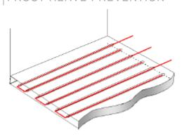
The substrata of freezer floors will withstand cold temperatures for a period of time, however if the ground temperature will eventually drop below freezing. At that point if water is present in the substrata frost heave of the freezer floor will occur. If severe, this will damage the foundation slab with the formation of cracks.
