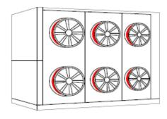
Fan cowlings on evaporator-blowers may 'ice up' and cause fan seizure.
