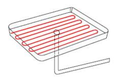
Drip trays are required to collect water droplets from the evaporator coils during defrost cycles.
